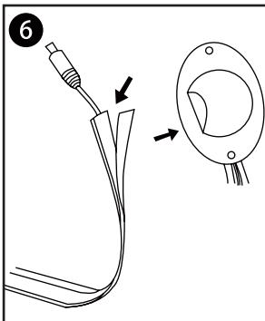
**Installation under the bed** Place the connected components under the bed. To ensure that the adapter is plugged into a power socket, otherwise, add an extra power socket. Before installing the sensor and strips, please tear up 3M tape adhesive protection layer. See figure 6.
